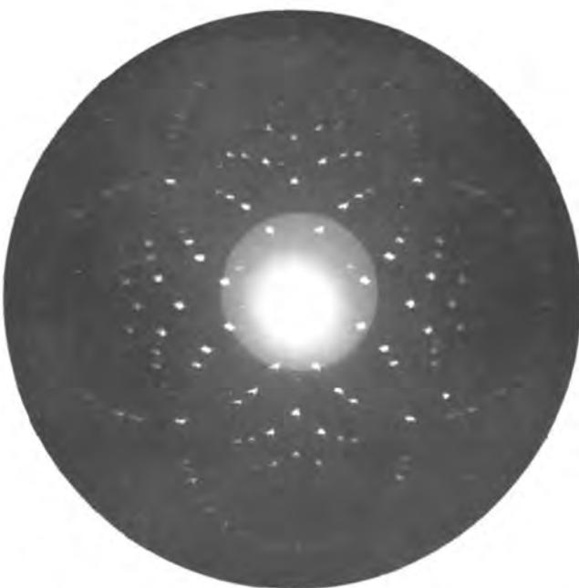
Fig. 1a. *X-ray Pattern of  $D\text{-}\{\text{Pt (l-Cptn)}_2\}\text{Cl}_2$  perpendicular to  $\{001\}$ ;*
